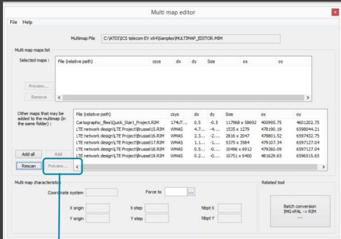
HTZ enables to use and manage different maps (DTM, clutter, images...) using different resolutions (e.g 2m, 10m, 50m, 100m...) and allows the users to use and switch between maps in a single scenario. As long as multiple raster resolution topographic maps are loaded, the software will support the multimap display depending on the zoom levels.
