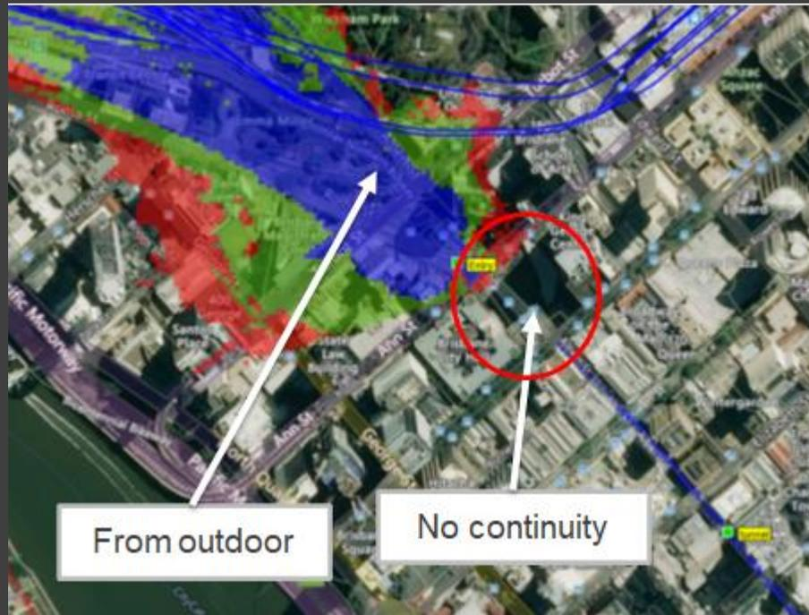
Composite coverage between outdoor and indoor (tunnel) coverage which creates the coverage continuity
